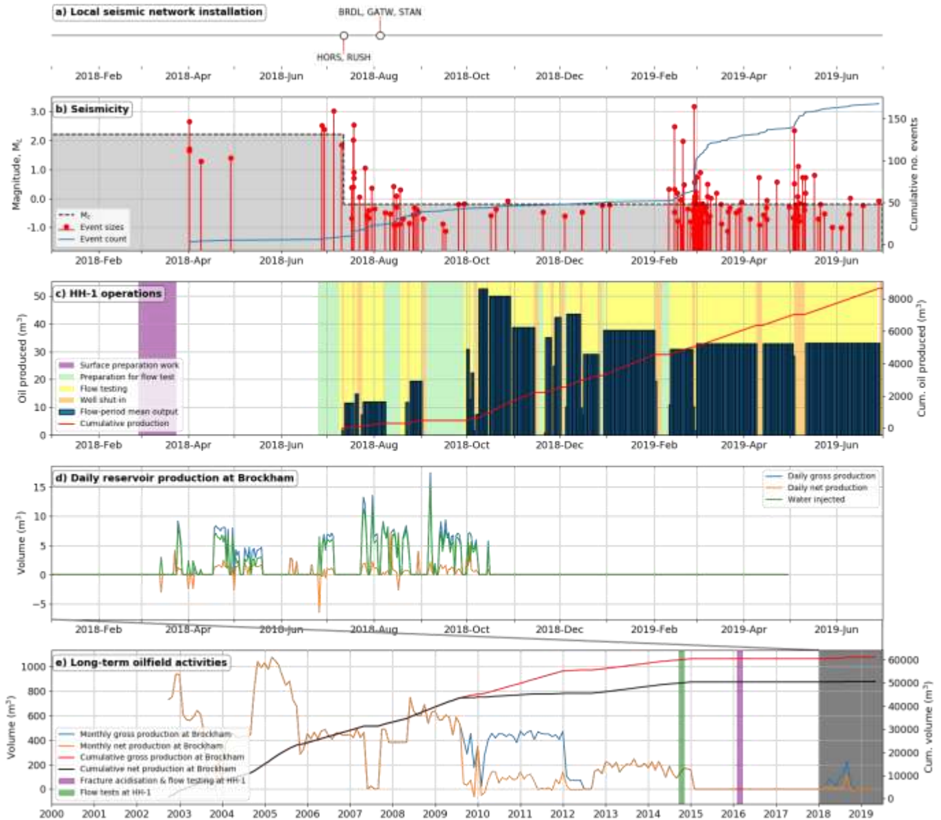
Figure 1: Timeline comparing evolution of the Newdigate seismic swarm with nearby oil field activities. (a) Installation dates of the 28 local temporary seismic monitoring network. (b) Detected seismicity, cumulative number of events, and the gray shaded area indicating the approximate completeness magnitude of the catalog over time. (c) Horse Hill-1: operations timeline (shaded boxes; see Table S4) together with flow-period averaged production and cumulative production over time. (d) Daily reservoir production and injection values at Brockham. (e) A long-term view of operations, with the time interval shown in panels above covering the 2018–2019 period delineated by the gray box and connecting lines.
