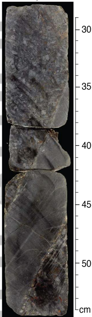
Figure 10. Hole U1473A diabase dikes with intrusive contacts: a. 5-cm thick granoblastic diabase dike intruding medium-grained subophitic olivine gabbro. Grain size fines toward dike contact with thin felsic zone along contact. Note the thin layer of white felsic material along the contacts. b. Granoblastic diabase dike margin in contact with olivine gabbro and tonalite interpreted as contact anatexis of the gabbro, with photomicrograph in cross polars of the tonalite-diabase contact. c. Granoblastic diabase in ragged reacted contact with gabbro. Note what appears to be a partially assimilated gabbro patch in the diabase in the plane-polarized light microphotograph where the gabbro and the diabase are in contact. Note that clinopyroxene is replaced by brown amphibole in the crystallization sequence, likely due to diffusion of water from the gabbro into the dike.
