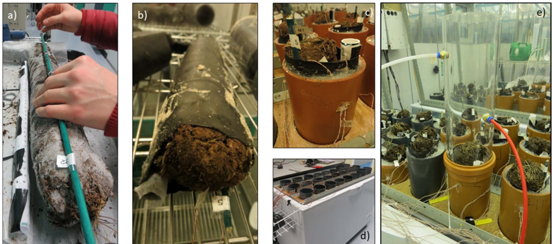
Figure 2. Experimental set-up of the experiment, including (a) the installation of the thermocouples across the soil profiles, (b) the protection of the cores inside heat shrinks, (c) the installation of the cores inside PVC pipes, (d) the refrigerated enclosure, and (e) the cuvette used for the gas flux measurements.
