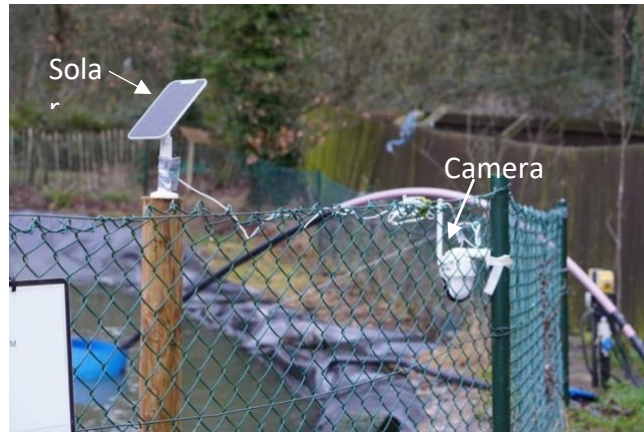
Figure S2 (Right): Reolink Go PT Plus (Reolink, China) in Nursery pool (camera 3). Camera is attached to the pole using supplied strap. Solar panel charges the camera and is placed in a place that will get direct sunlight to be able to charge the cameras.
