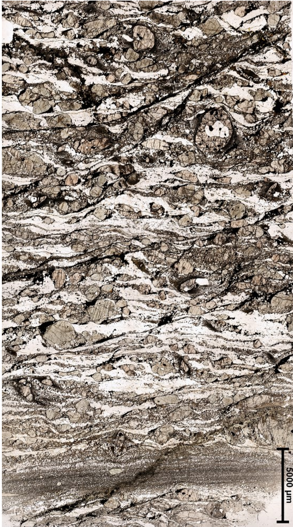
Sample F32A: amphibole-poor metagabbro (upper portion), mylonite. Amphibole-rich metagabbro (lower portion), ultramylonite. Scale bar 5mm.
