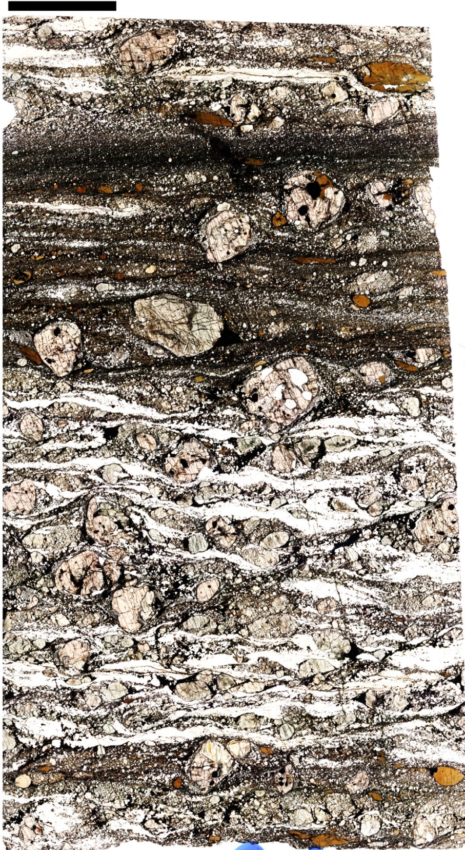
Sample F20A: amphibole-rich metagabbro (upper portion), ultramylonite; amphibole-poor metagabbro (central portion), mylonite; amphibole-rich metagabbro (lower portion), ultramylonite. Scale bar 5mm.
