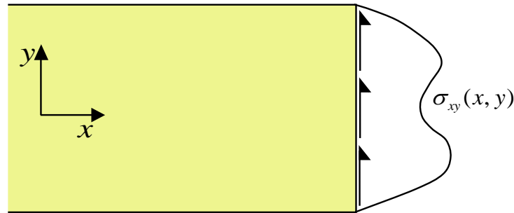
Figure 3: Shear stress distribution across a beam [9].
