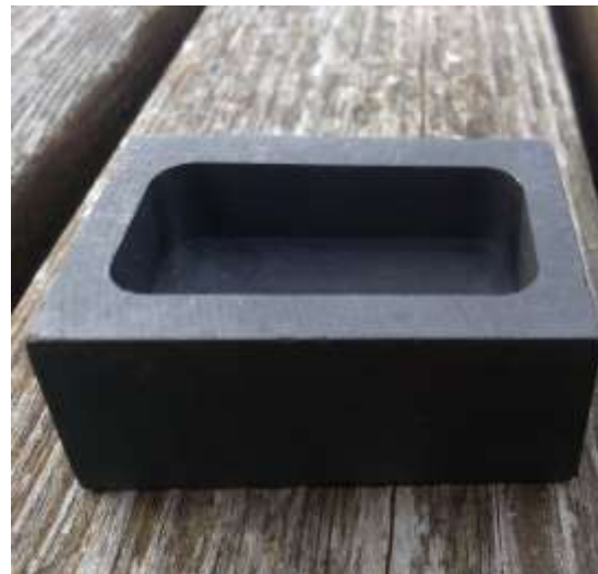
Figure 2: Graphite mold used for gravity casting the ingots
