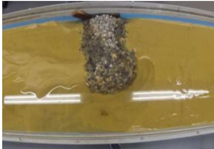
Figure 13: Image of Falmouth model post-test indicating smooth upstream bed material
