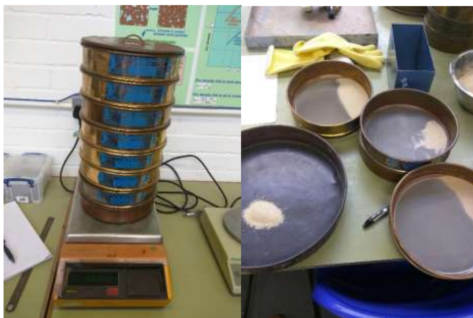
Figure 2: a) Sieve test apparatus b) Individual sieves showing collected bed material post-test.
