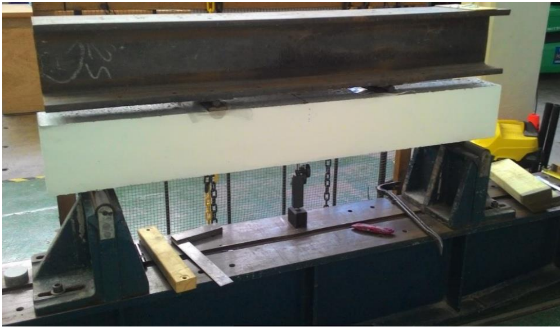
Photo 5: R.C. Beam Two-Point Load Setup.
