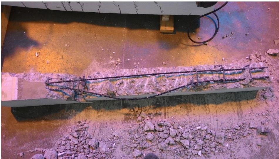
Photo 9: Bottom basalt rebar elongated.
