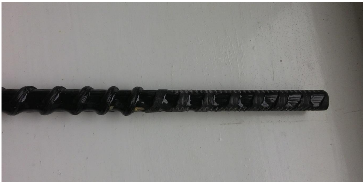
Photo 2: Ends of BFRP Rebar Sanded Off.
