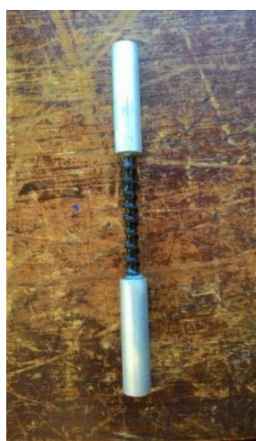
Photo 1: BFRP rebar encased in threaded aluminium rods.
