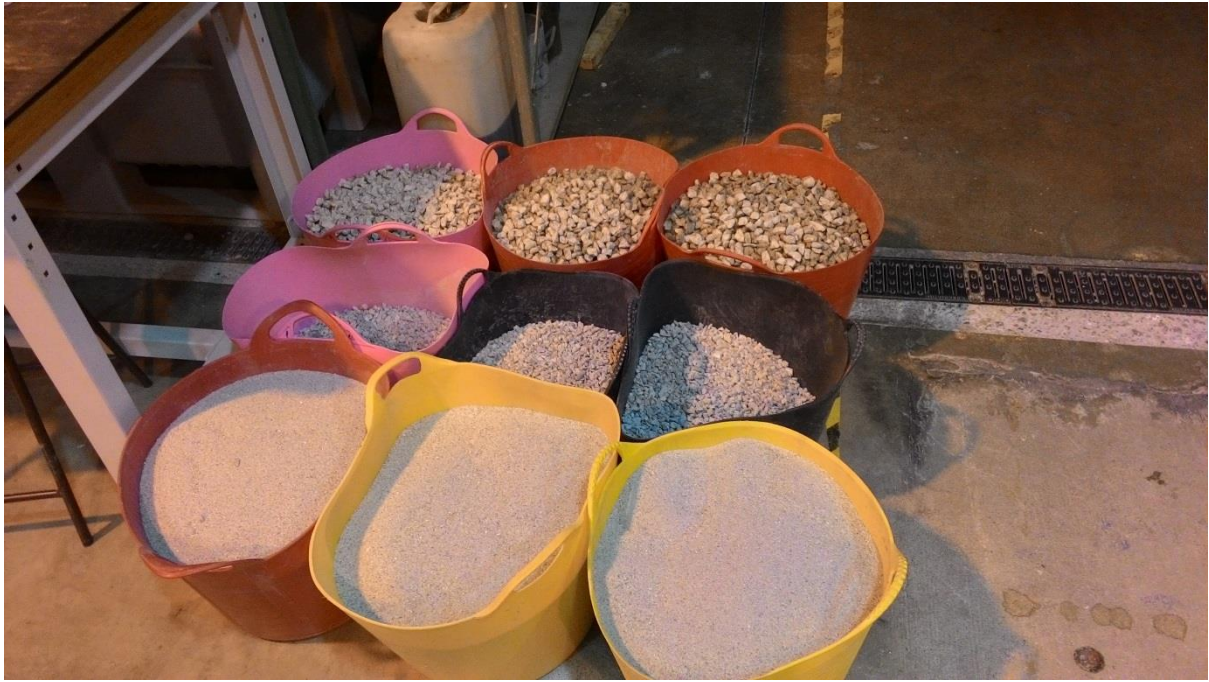
Photo 6 –Aggregate Quantities for Concrete Mix.
