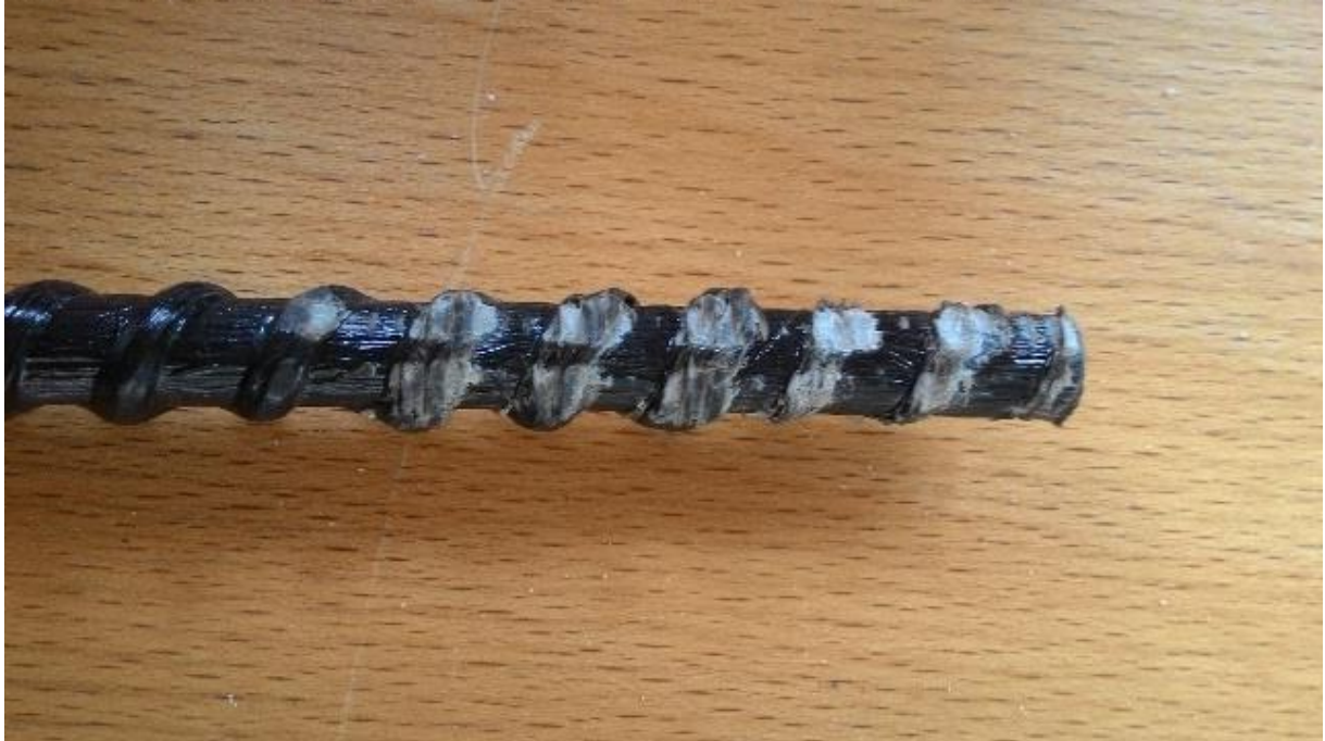
Photo 1 – BFRP Rebar Sample Ends Sheared Off During Tensile Strength Test.
