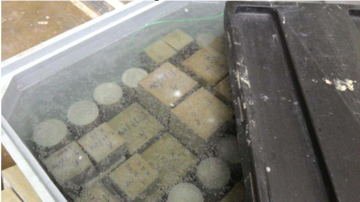
Photo 10 – Concrete (C28/35) Concrete Cube Curing Inside the Water Chamber.
