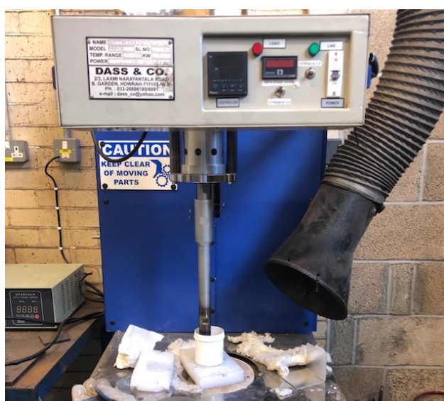
Figure 5: Ultrasonicator dispersing CNT/PDMS.
