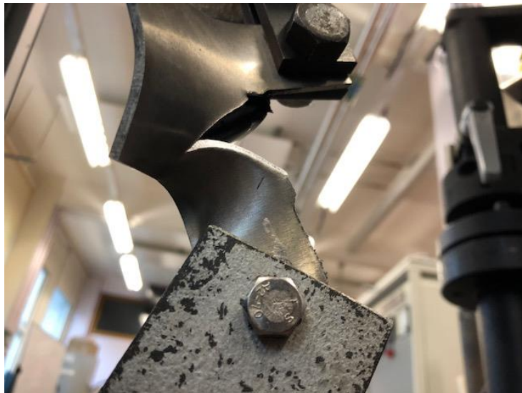
Figure 14: Crack behaviour on the aluminium sample.
