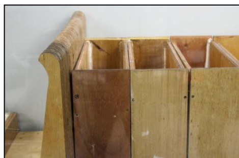
Figure 37: Gaps between collection buckets
