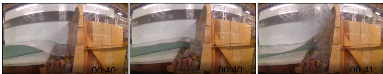
Figure 19: 0.7Hz at 0m/s wind showing an uprush of aerated water with added time stamp
