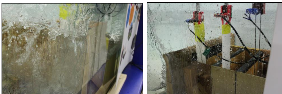
Figure 30: Friction from the side walls affecting incoming waves
