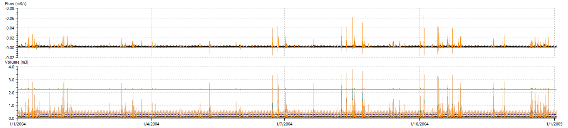
Figure 22: Conduits where only potential green roofs drain into it (green roofs present)
