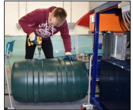
Figure 29: Drilling holes for pipe attachments
