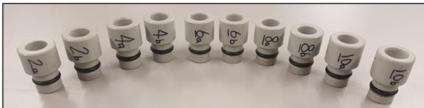
Figure 6: 2mm, 4mm, 6mm, 8mm, 10mm orifice inserts
