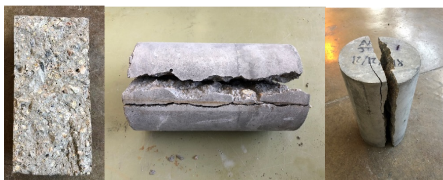
Figure 15: Reference mix sample 1 after splitting tensile failure
