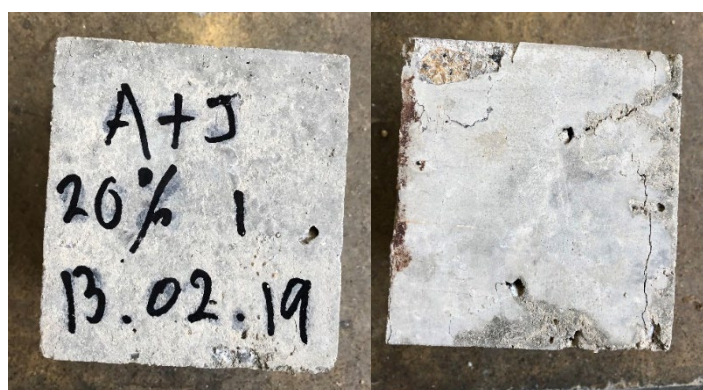
Figure 13: 100 mm 3 20 % sample 1 – after compressive strength testing
