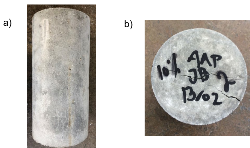
Figure 16: 150 \varnothing mm x 300 mm samples after splitting tensile failure a) 20 % replacement sample 1 b) 10 % replacement sample 2
