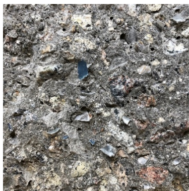
Figure 9: Concrete beam with 20 % plastic
