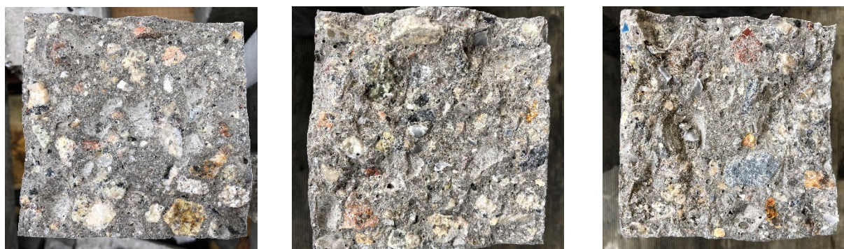
Figure 19: Concrete beam samples split open after flexural strength testing
