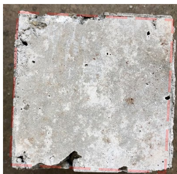
Figure 8: Concrete cube sample
