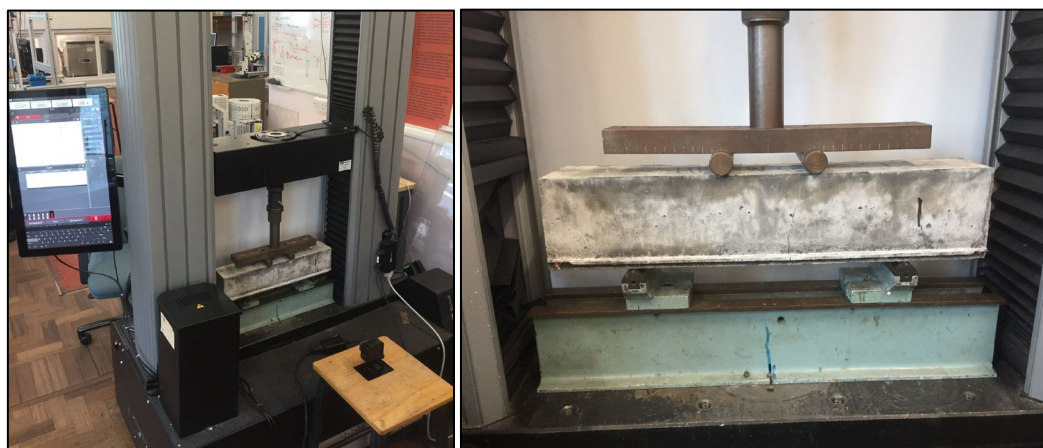
Figure 24: (left) - Instron machine used for flexural test Figure 25: (right) - Beam undergoing flexural test
