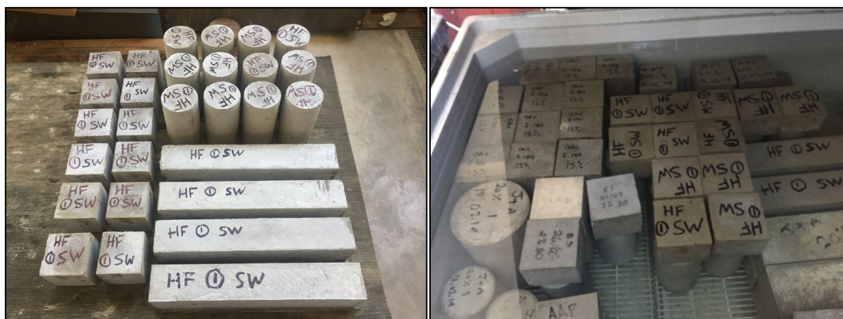
Figure 16: (left) - Samples after unmoulding Figure 17: (right) - Samples placed in curing tank
