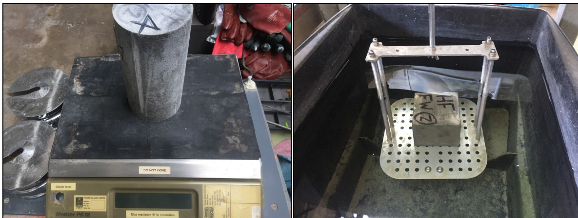
Figure 18: (left) - Sample being weighed dry Figure 19: (right) - Sample being weighed in water
