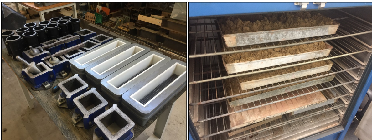
Figure 13: (left) - Samples prepared and ready for mix Figure 14: (right) - Sand being oven dried
