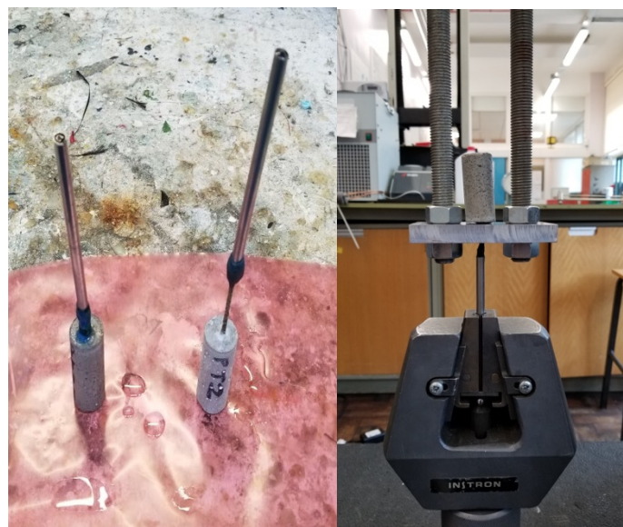
Figure 12: Carbon Fibre Tow Specimen Embedded in Concrete Cylindrical Matrix (Left) Pull-Out Test Set-Up (Right) Reproduced with kind permission from Ji (2019)
