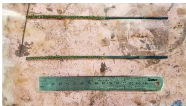
Figure 11: Sand Treated Carbon Fibre Tow Reproduced with kind permission from Ji (2019)
