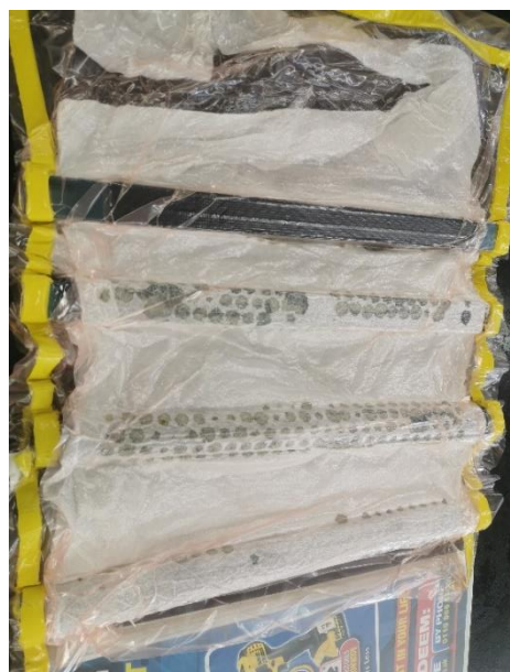
Figure 16: 'Chain Linked' Prepreg Wrapped Tubes in Vacuum Bag
