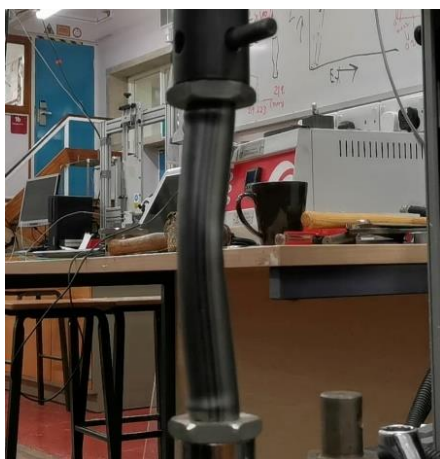
Figure 26: Global Buckling of 200mm Specimen P200R1
