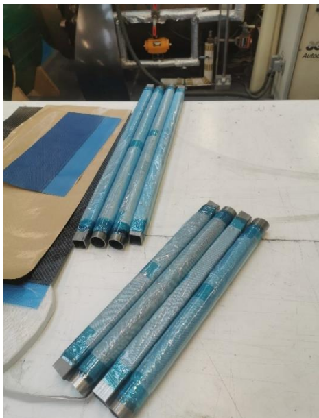
Figure 15: Application of Peel Ply and Release Film
