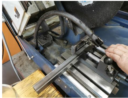
Figure 8: Using Abrasimet Cut-Off Saw for Accuracy
