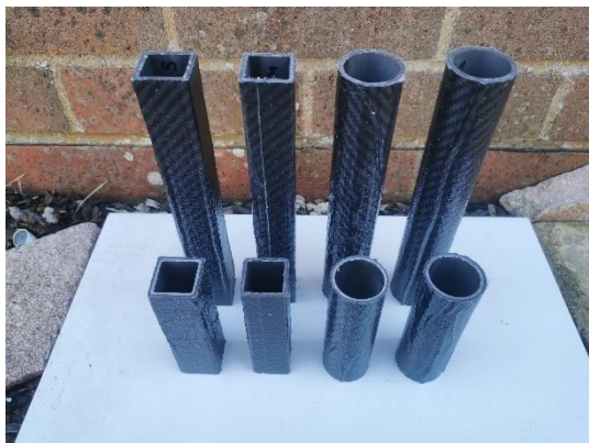
Figure 17: Composite Clad Steel Tubes Cut to Length
