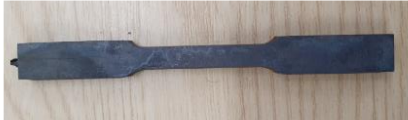
Figure 2: Tensile test specimen after manufacturing.
