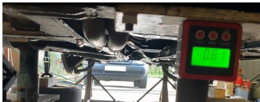
Figure 24: Position 11 twist measured directly off fixture plate
