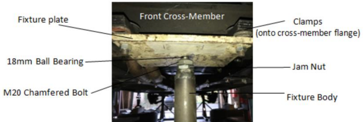
Figure 20: Front fixture detail
