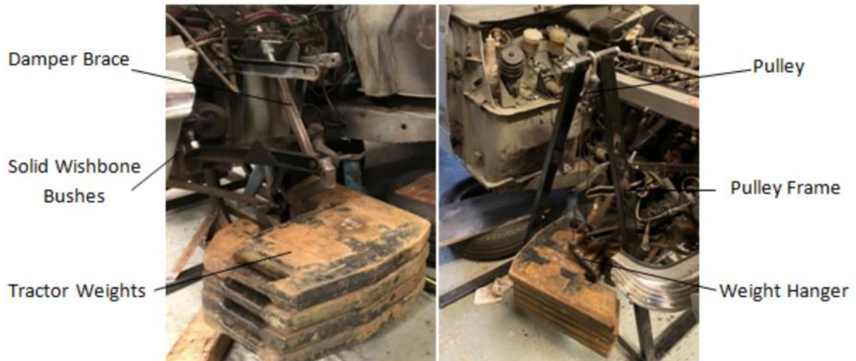
Figure 21: Left and right front corners respectively, in test configuration
