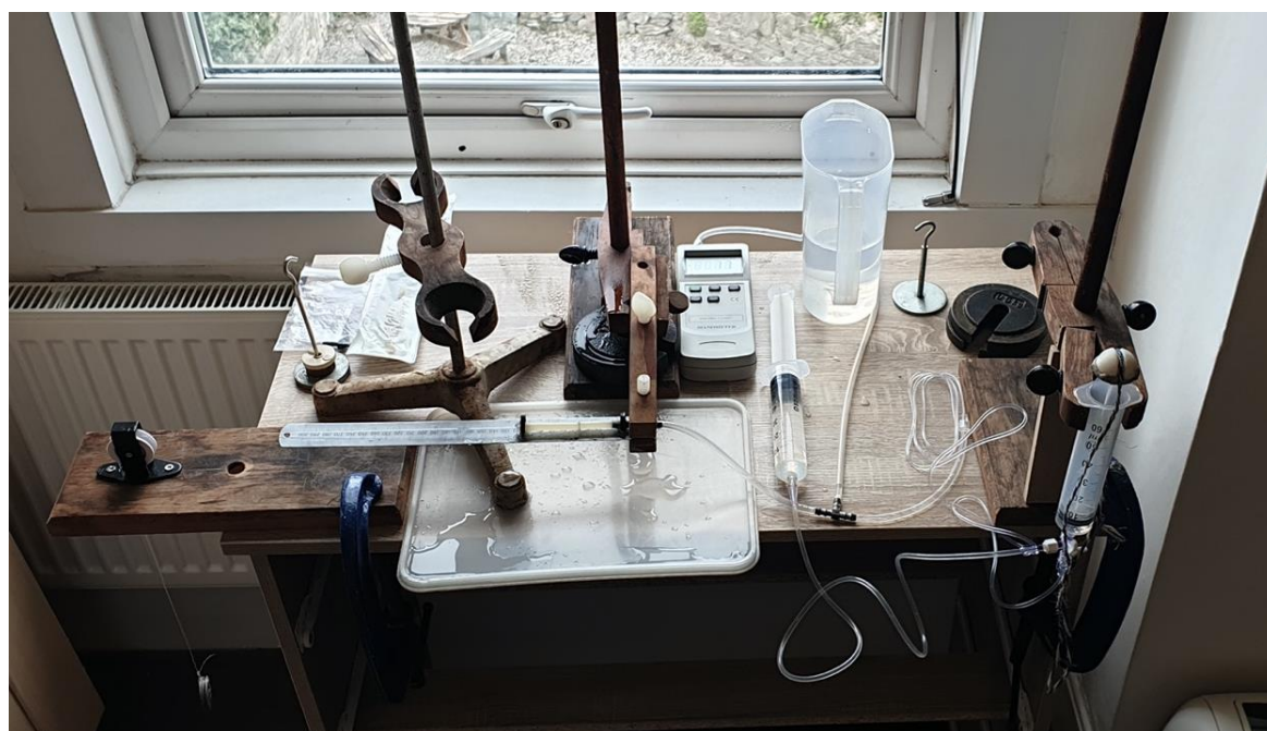
Figure 12: Rig set up for Optical Method – Same as CT set up with addition of clamp to hold camera and steel rule for calibration. 3-way syringe valve also pictured.
