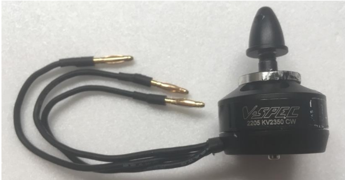
Figure 6: Vspec 2205 2350kv 420W brushless motor
