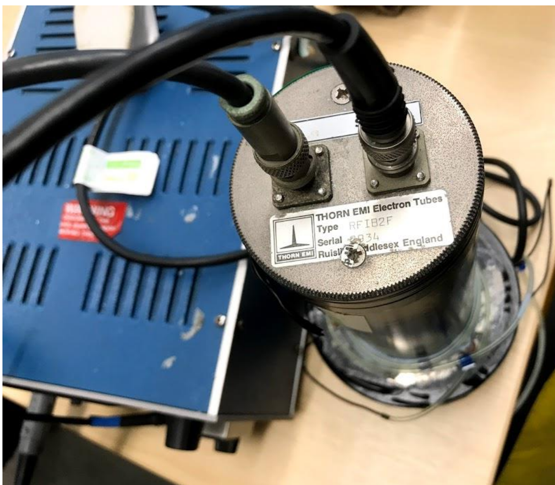
Figure 4: A photomultiplier tube
