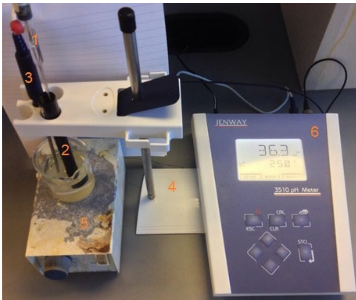
Figure 5: Experimental setup for proof of concept laboratory work. The figure shows the Mettler Toledo electrode (1), the ThermoFisher Orion 9512 electrode casing with ammonia selective membrane and filling solution (2), the thermometer (3), the electrode stand (4), the magnetic stir bar (5) and the Jenway 3510 pH meter (6).
