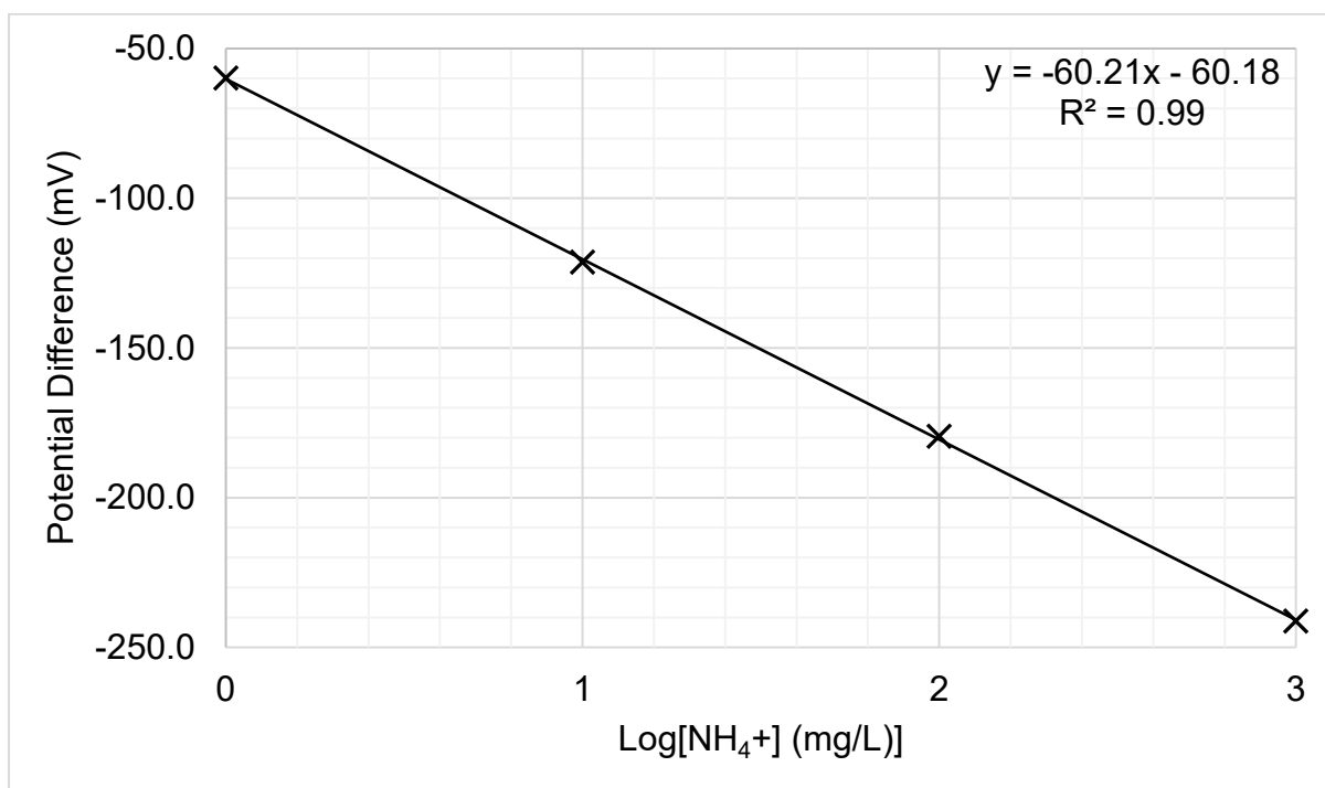
Figure 11: CSM electrode calibration graph in Fe(III) bioleaching solution calibration solutions.
