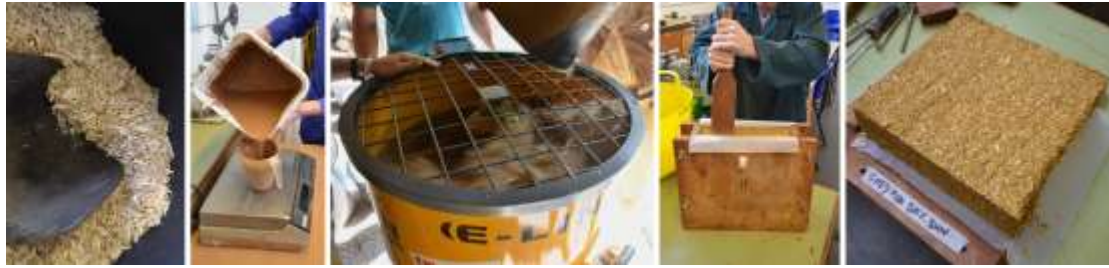
Figure 1. Sample preparation stages. (left to right. Cut fibre, weighed slip, mechanical mixing, hand tamping, completed sample)
