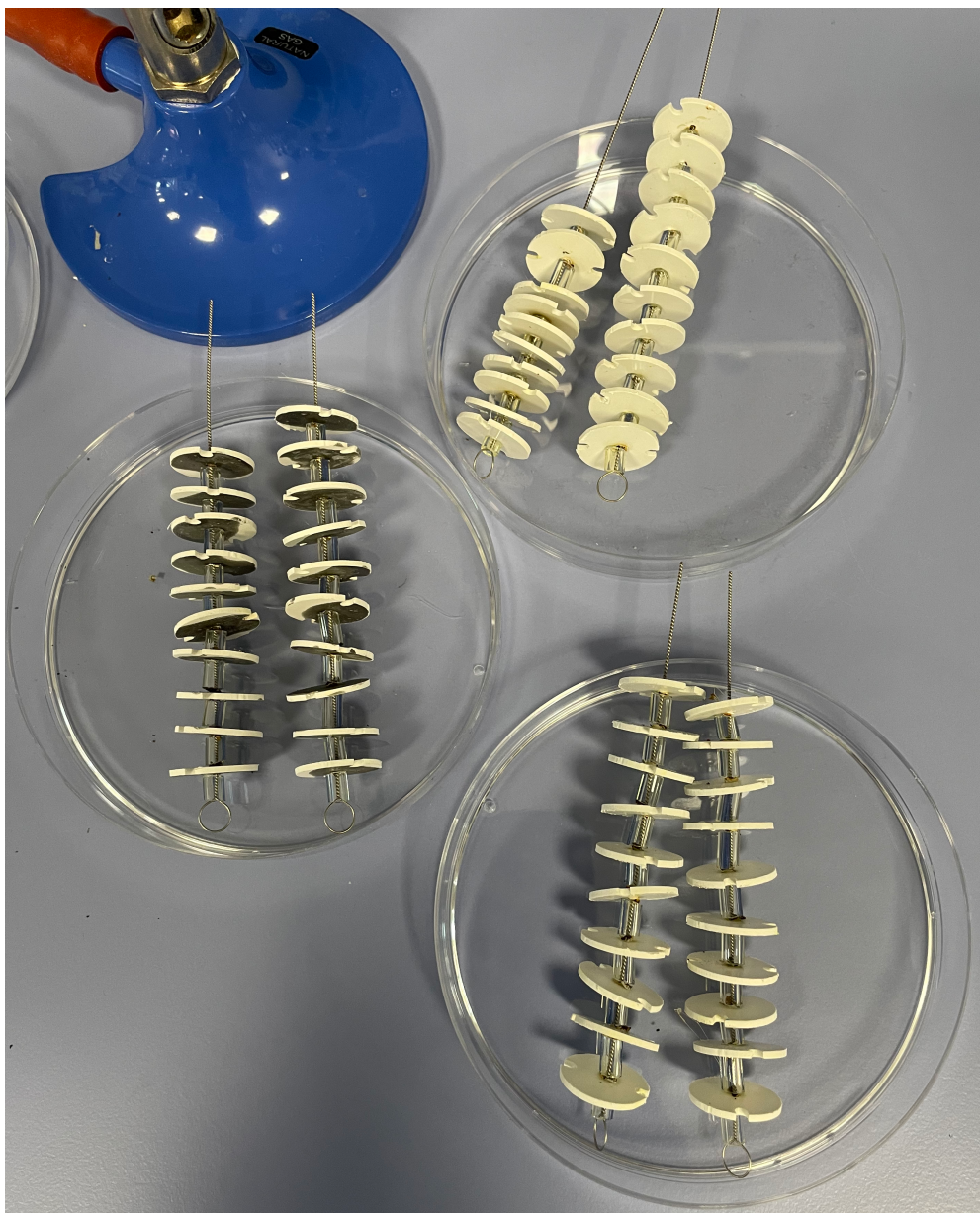
Figure 5.2: Appearance of uPVC discs with different surface finishes mounted on nichrome wires with plastic spacers between discs to facilitate separation.
