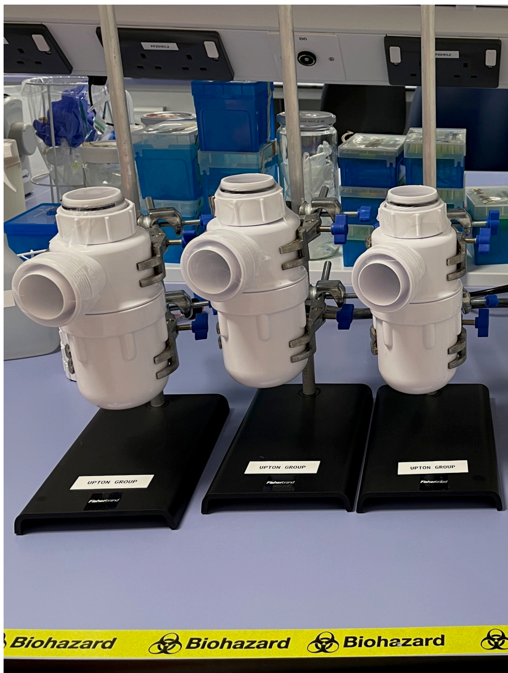
Figure 5.3: Setup of the laboratory benchtop sink trap model system. Bottle-style sink traps were assembled and set up on retort stands on a laboratory bench with their inlet and outlet ports sealed with parafilm.
