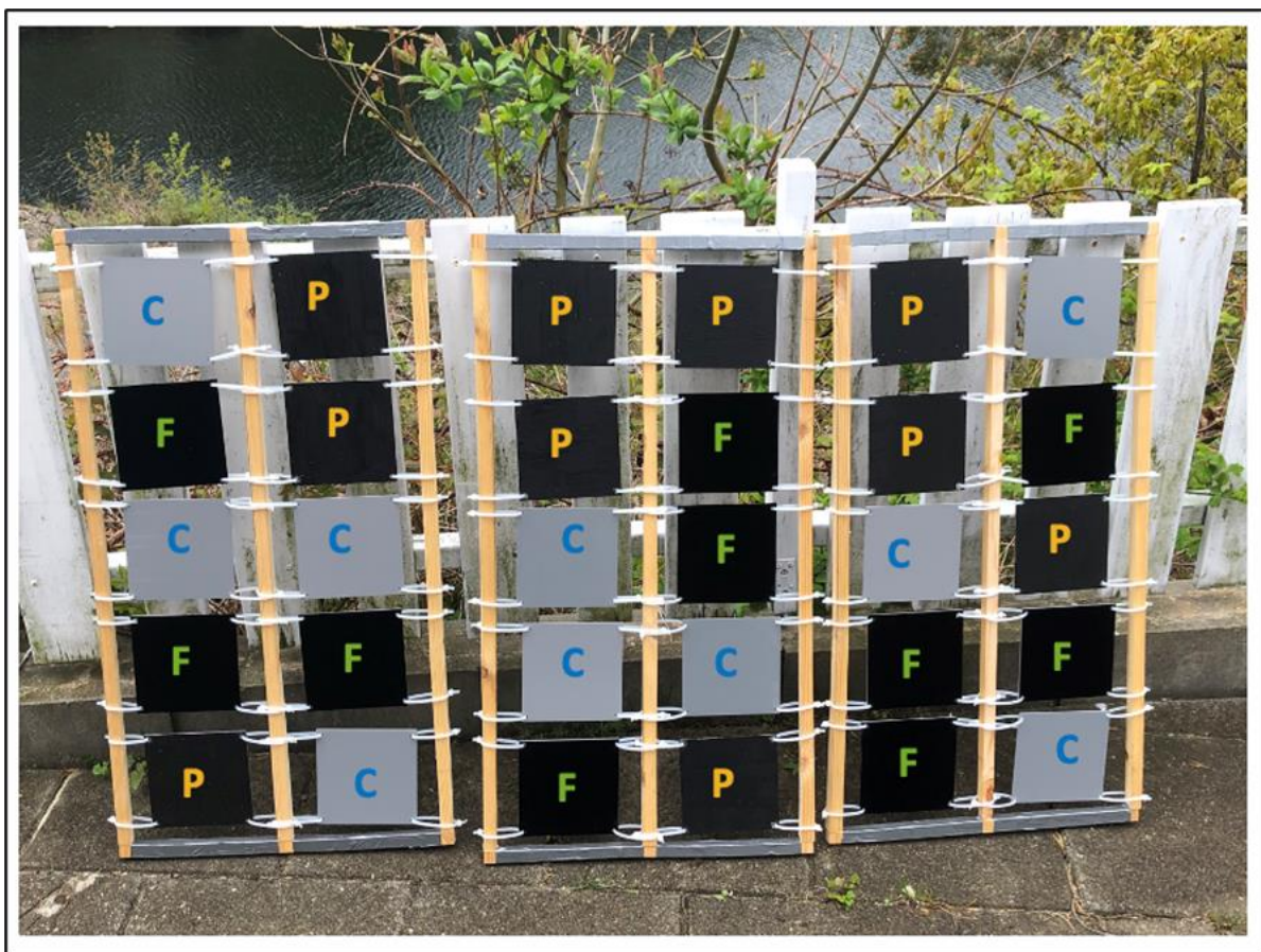
Figure 2: Three wooden frames for the dock experiment included 10 PVC panels for each treatment: C= control, P= paint, and F= fibre.
