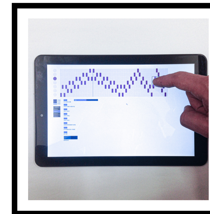
Figure 3. Haplós controller and sequencer. Patterns and pattern playback speed can be adjusted on the fly.
