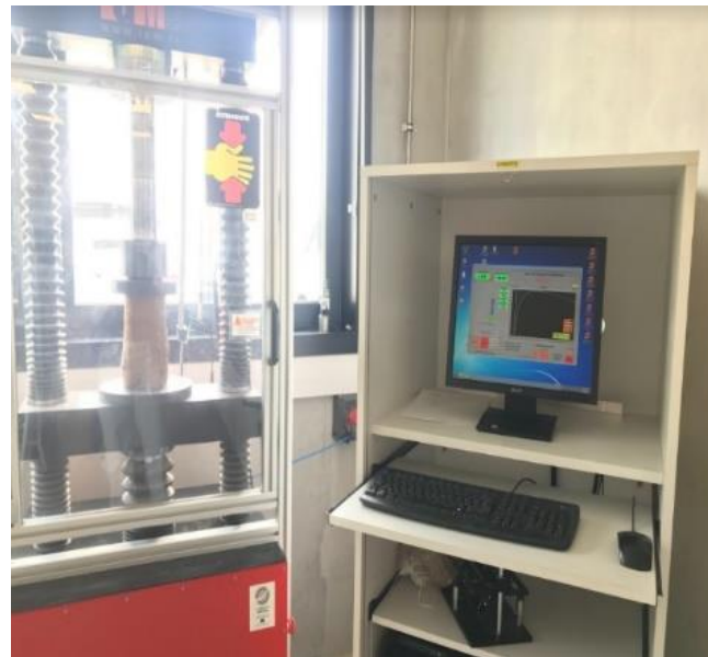
Figure 4. Compressive strength test on cob samples at different water content under an IGM press.
