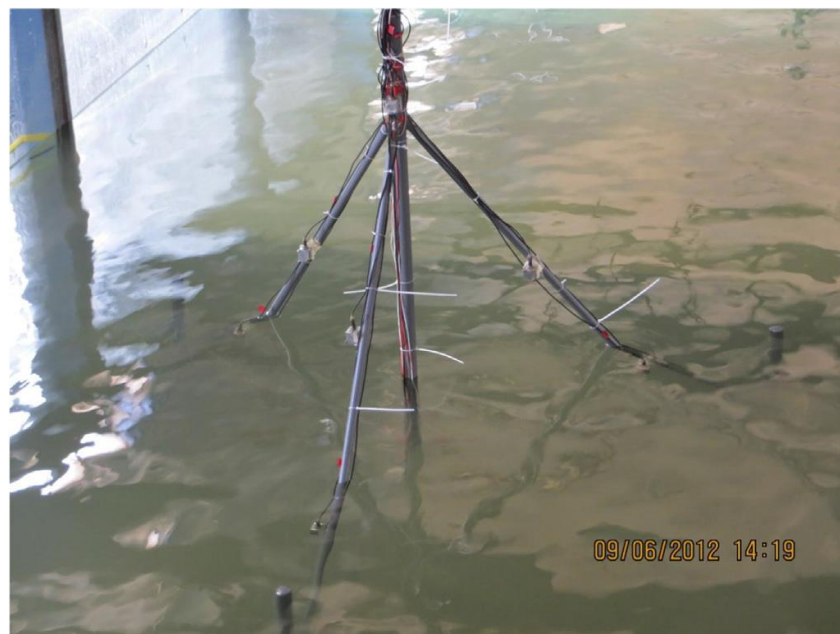
Figure 2.4 Experimental model (1:15 scale) of a jacket-type foundation (Liu et al., 2014)
