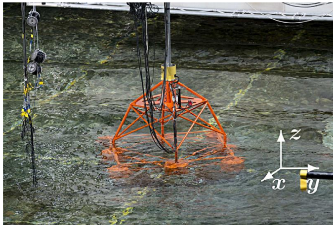
Figure 2.5 The 1:37 scaled TLP platform ( Adam et al., 2014 )
