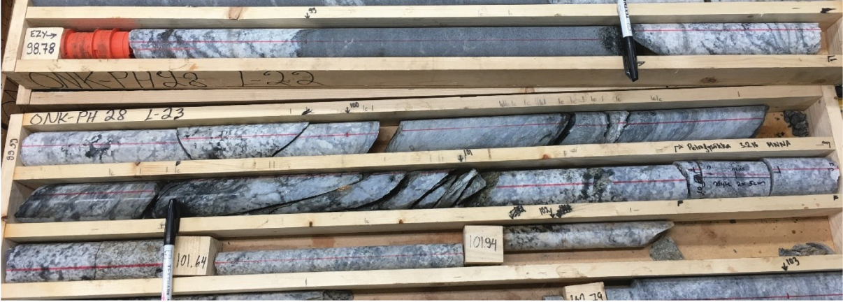
Figure A 4 Photo of selected dill cores. Core section from horizontal drill core ONK_PH28. Photo shows the extracted core length at the 98.78- 102.13 m distance from the start of the drill core
