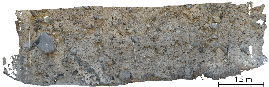
Figure B.1: Orthophoto generated from 3D model for the large scale of the outcrop at locality 2. The 3D model was generated with 245 photographs taken in the field and covers an area of 21 m 2 , with a resolution of 0.21 mm/pixel.
