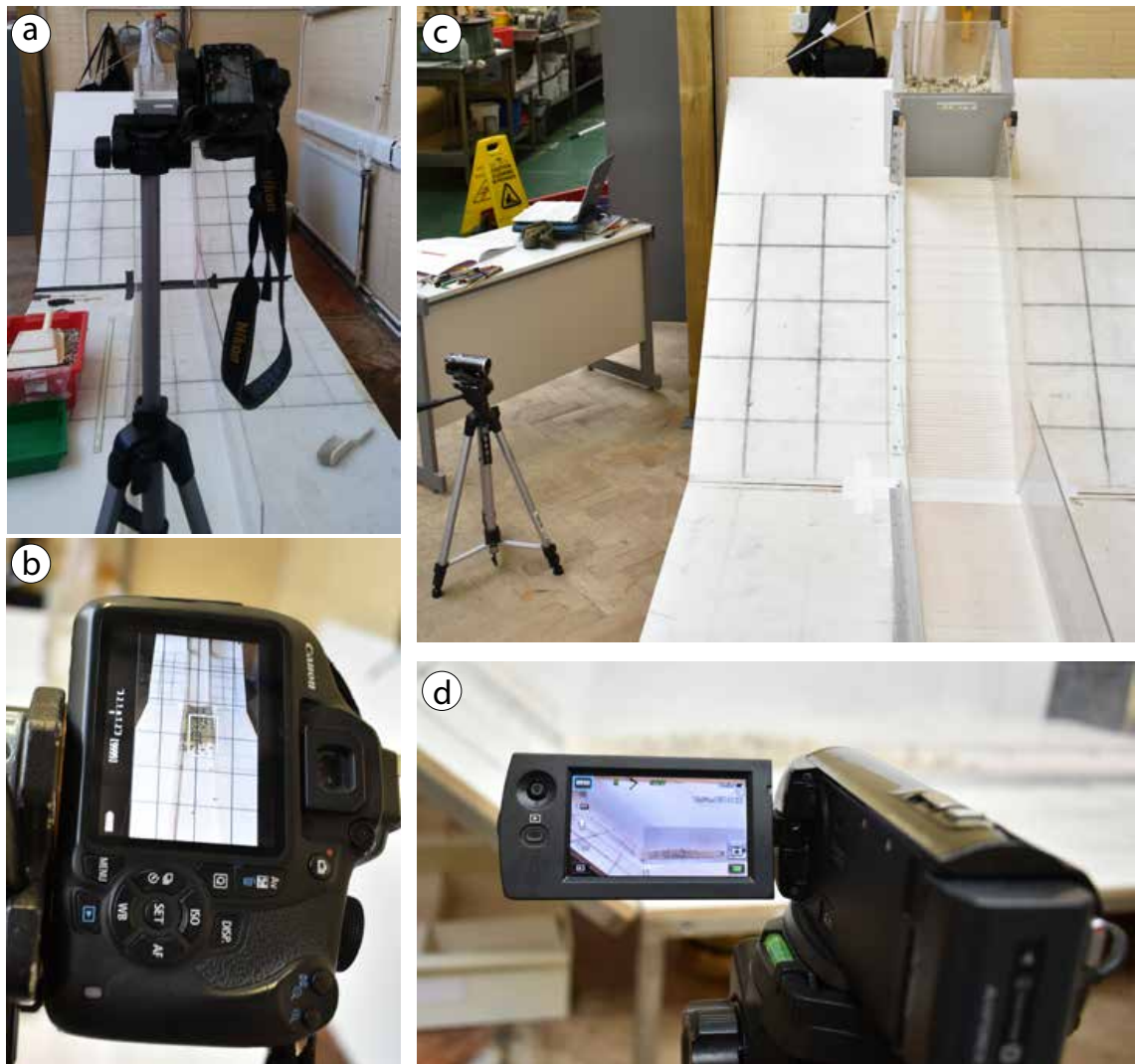
Figure 6.3: Camera setup during the experiments. A Frontal camera placement. B Frontal camera frame view. C Lateral camera placement. D Lateral camera frame view.
