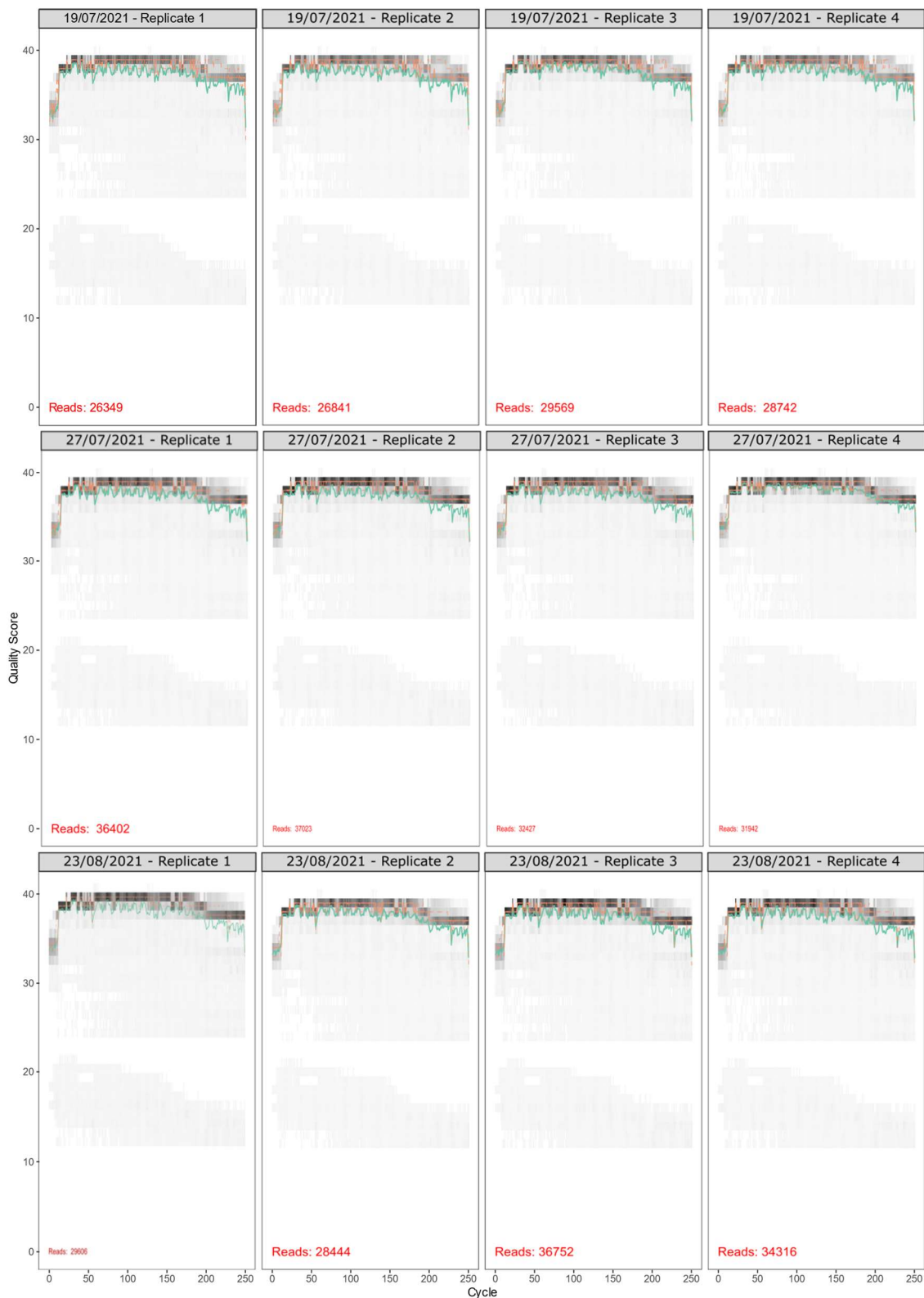
Appendix Figure 14. E) Quality profiles for each of the 16S rRNA samples (forward reads) produced by Illumina MiSeq sequencing. Quality profiles were produced using the DADA2 pipeline (Callahan et al., 2016) and visually inspected to ensure all samples were of sufficient quality before continuing with subsequent analysis. Each sample is labelled with the date the sample was collected and replicate number.
