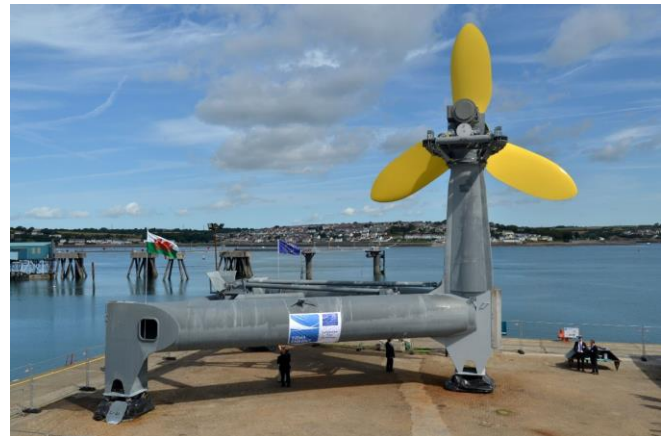
Fig. 1. Tidal Energy Limited ‘Deltastream’ device prior to deployment in Ramsey Sound. Source [3].
