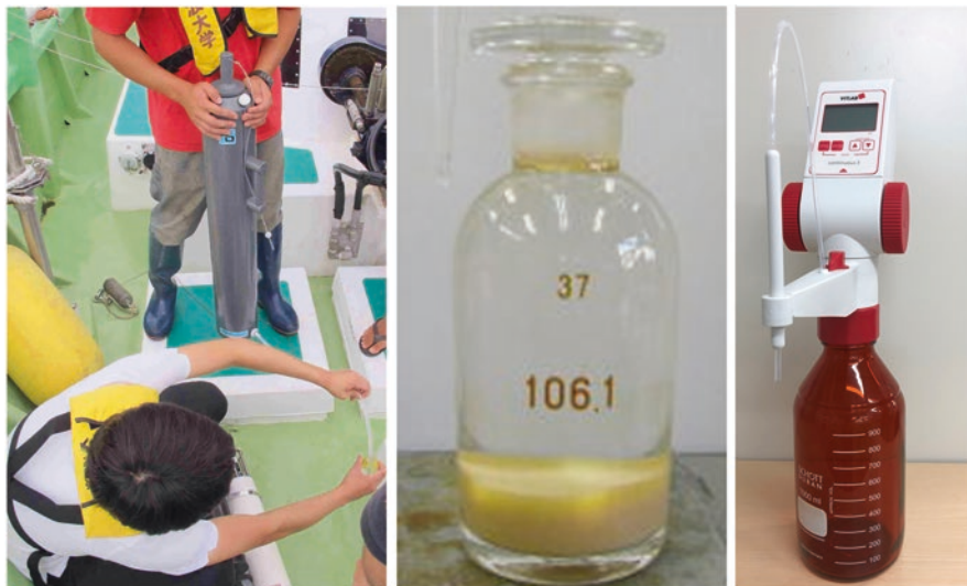
Fig. 25.1 Procedures for DO analysis. Collection of seawater, precipitation after the addition of reagents 1 and 2, and the digital burette for titration
