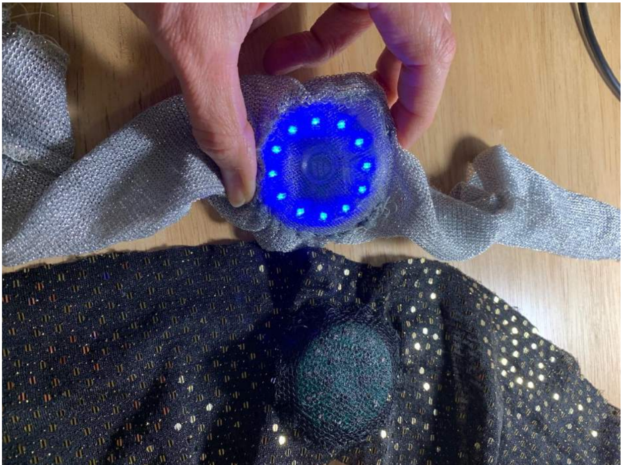
Figure 5.15: Sounddrop devices embedded into fabric bands (Hurban, 2022)
