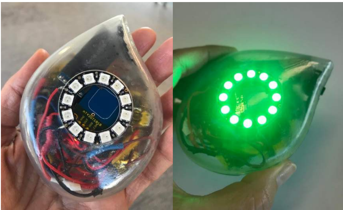
Figure 5.7: Clear/transparent resin for 3D printed casing (Hurban, 2021)
