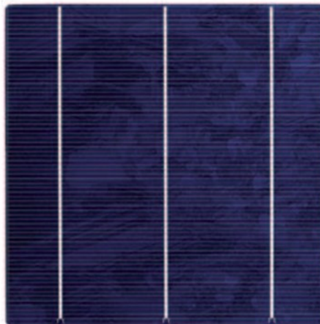
Figure 2- 12 Optical image of a polycrystalline Si solar cell with screen-printed contacts [40].
