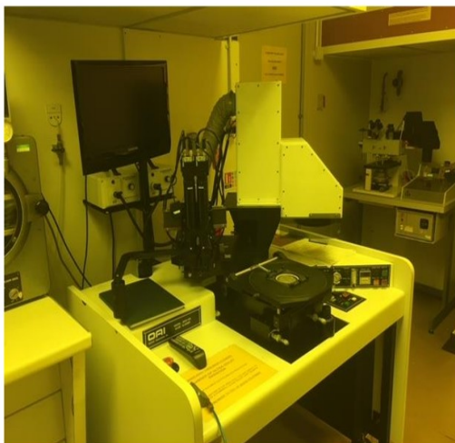
Figure 3-7 An optical view of the mask aligner in the cleanroom (left). An illustration showing the photolithography and lift-off processes (right), (a) A spin coating is used to apply a layer of photoresist to a substrate. (b) Subjecting the area to UV light for a predetermined amount of time while wearing a mask with a predetermined pattern. (c) Eliminating the positive photoresist that has been exposed by applying developer. (d) The process of sputtering a layer (e) Processing the lift-off operation with the help of the remover.
