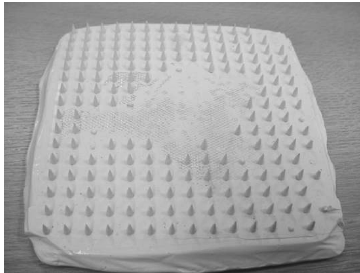
Fig. 3.13: Reinforced Ceramcor moulding showing flow issues caused by change in permeability
