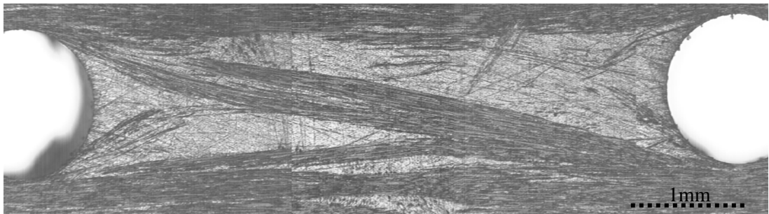
Fig. 5.16: Hole-to-hole fibre distortion from RFI mouldings
