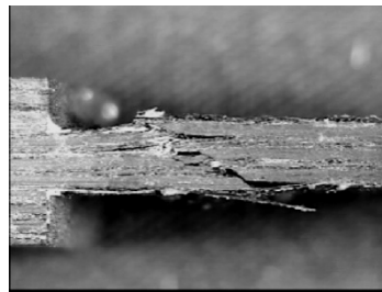
Fig. 4.25: RT moulded hole PP UCS failure
