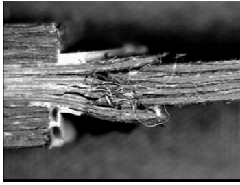
Fig. 4.30: H/W non-perforated PP UCS failure
