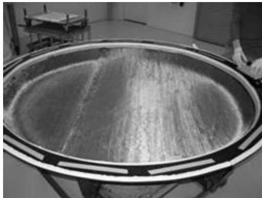
Fig. 8: Full ply on dome tool
