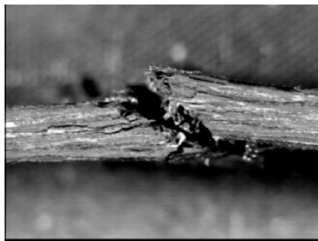
Fig. 4.24: RT non-perforated PP UCS failure
